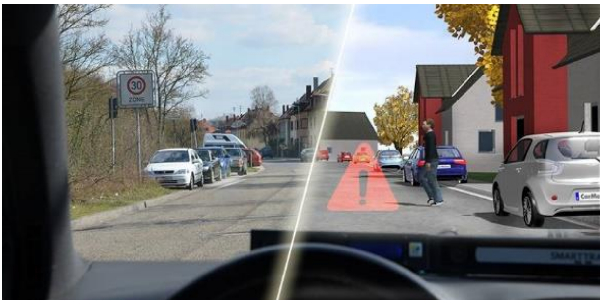
Testing an emergency brake assist system with the vehicle-in-the-loop method
