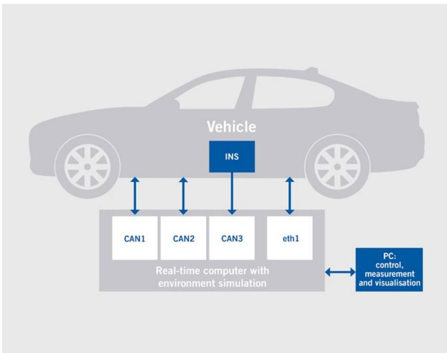
**FIGURE 3** Schematic outline of the vehicle-in-the-loop setup (© IPG, BMW)
