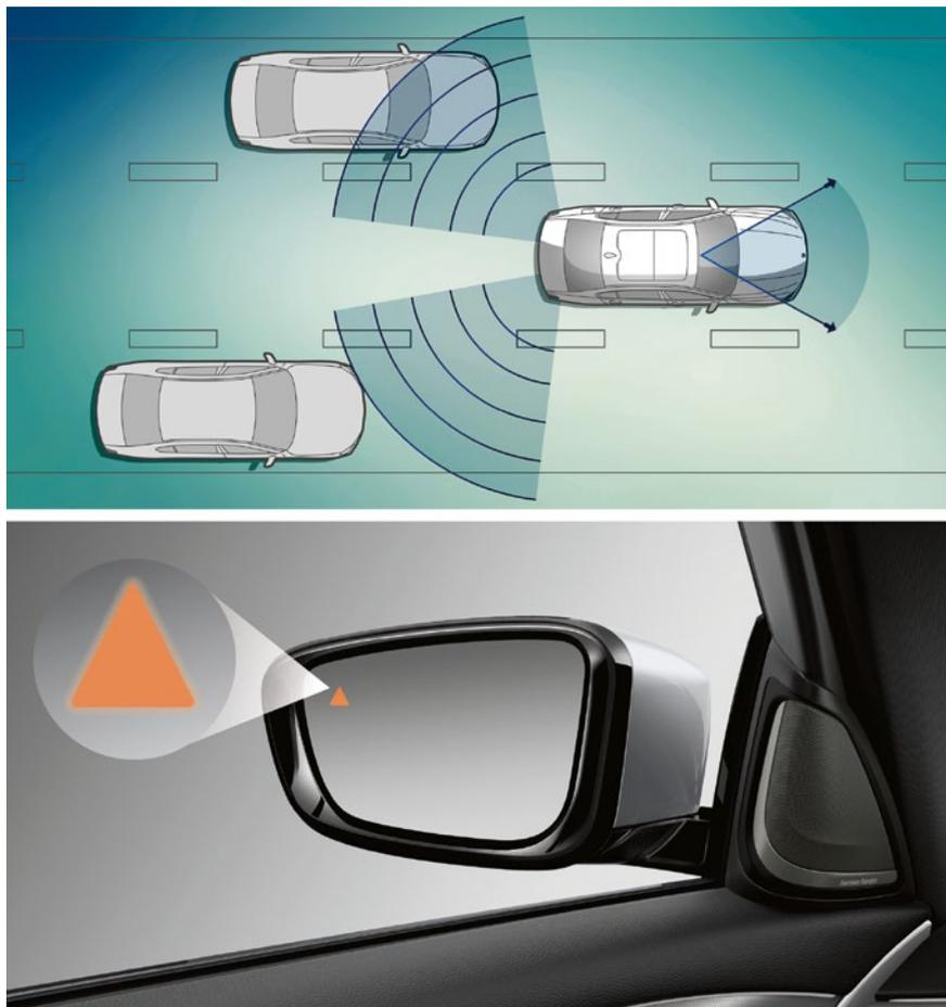
**FIGURE 1** Lane change warning: drivers are alerted to vehicles in their blind spot (top) via a warning symbol in their wing mirror (bottom) (© BMW)
