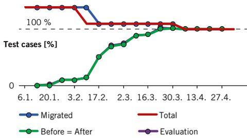
**FIGURE 3** Migration tracking of a specific test catalogue for a brake control function with standardisation to target test catalogue requirements (© EFS)
