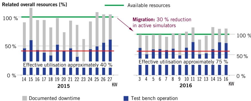
**FIGURE 4** Results of tool migration today: reduction in test benches, comprehensive tracking of test bench capacity, approximation to the optimal 85 % test bench capacity limit (© EFS)
