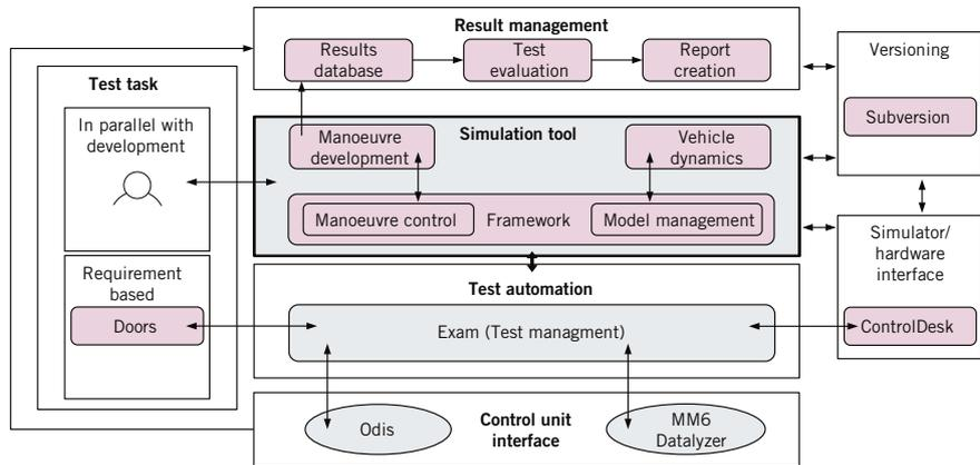
**FIGURE 2** Functional requirement and creation of a tool chain for fully automated validation of brake control functions on a hardware-based test bench (© EFS)
