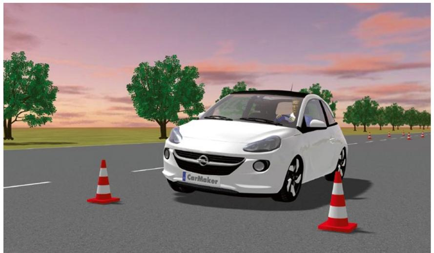
**FIGURE 1** Simulation-based homologation of ESC systems (© IPG)
