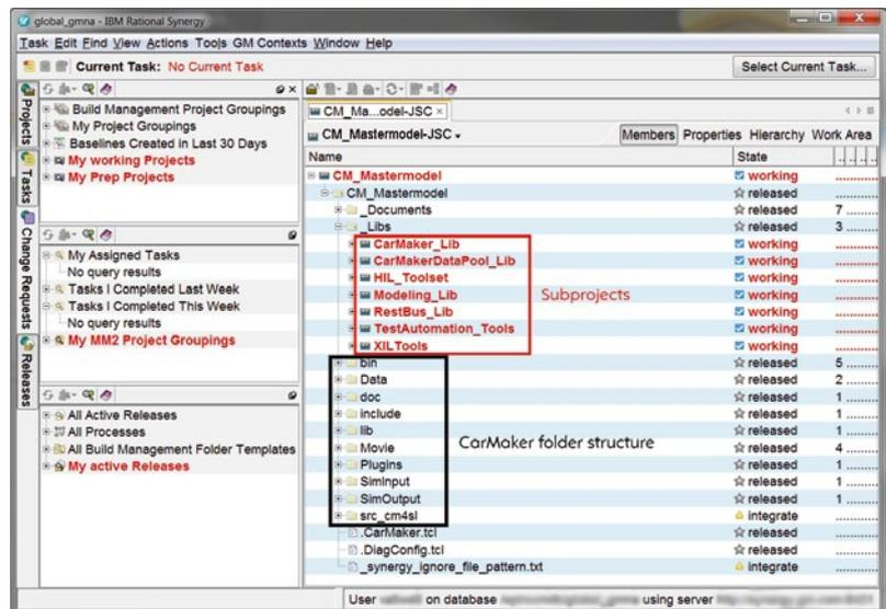
FIGURE 3 A global database is the golden source for all master model files and includes the configuration management as well as version control. The database project mirrors the CarMaker folder structure and includes several sub-projects (© Opel)
