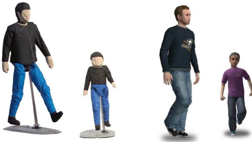
**FIGURE 1** Real Euro NCAP pedestrian targets (EPTa and EPTc, left) versus virtual pedestrians (adult and child) © Euro NCAP and IPG Automotive)
