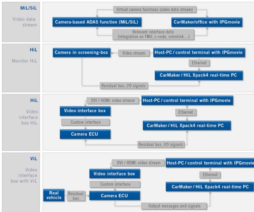
**FIGURE 3** Overview of the functional principles of the single tools (© IPG Automotive)
