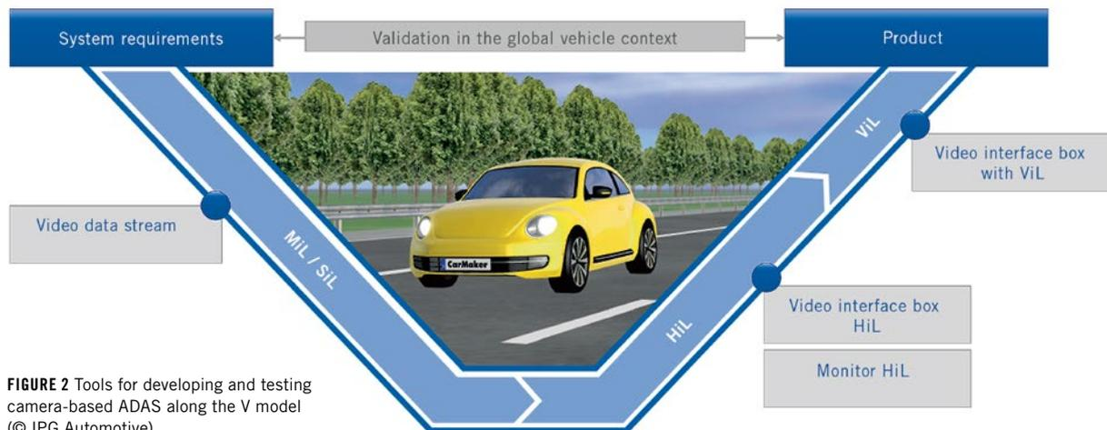
**FIGURE 2** Tools for developing and testing camera-based ADAS along the V model © IPG Automotive
