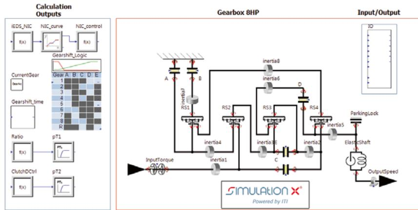
FIGURE 2 Screenshot of a SimulationX model of the automatic gearbox 8HP by ZF (© ITI)
