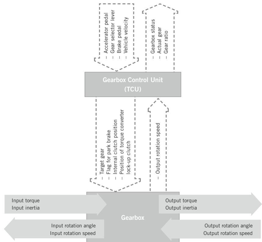
**FIGURE 1** Realistic interfaces with gearbox components are necessary for an easy and continuous integration; additional inputs and outputs can be included (© IPG)
