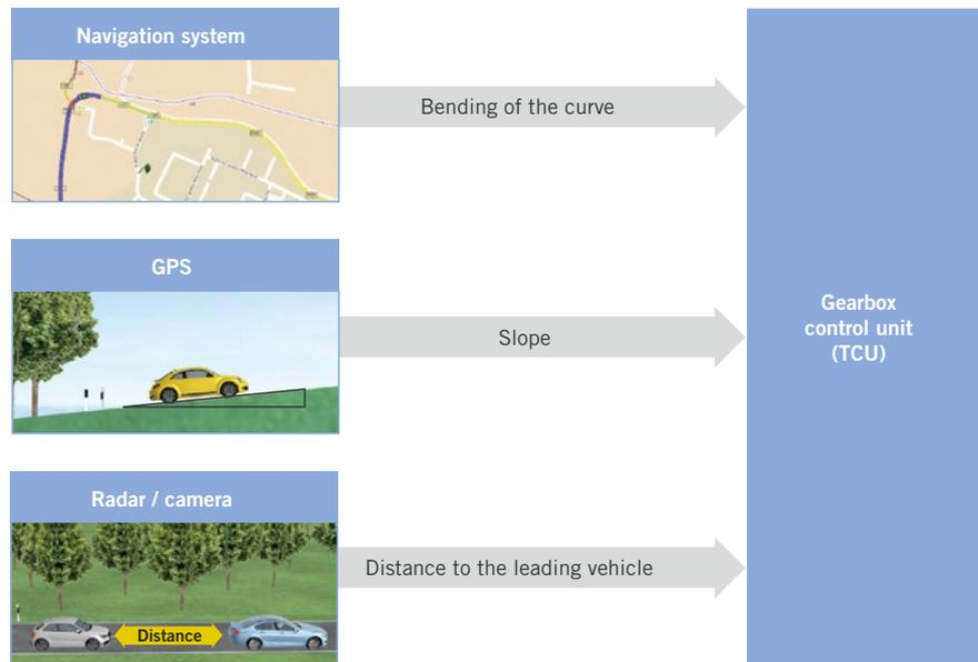
FIGURE 3 Information which is acquired by sensors and forwarded to the gearbox (transmission) software (© IPG)
