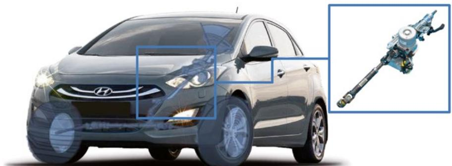
**FIGURE 1** Hyundai i30 with column-type electrically assisted power steering
