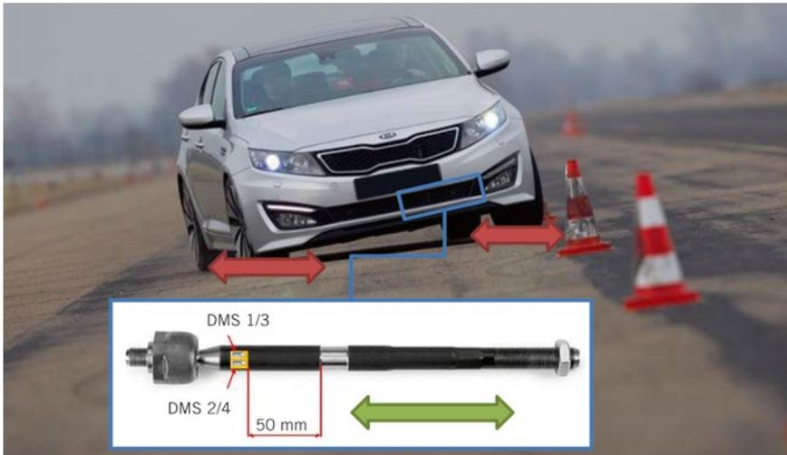
**FIGURE 2** Objective tests on the proving ground with steering rack force measurement via strain gauges (DMS) on the tie rods
