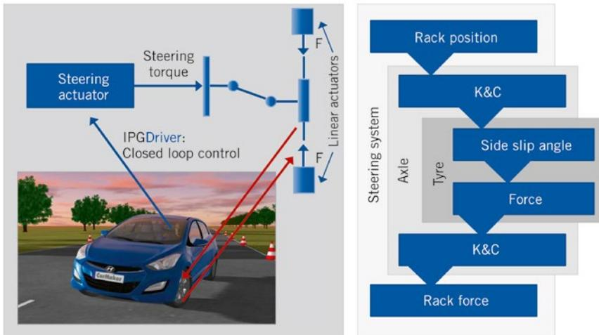
FIGURE 4 Hardware-in-the-Loop method for the steering system
