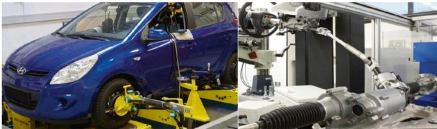
**FIGURE 3** Vehicle specimen (left) on the suspension measurement device in order to test elastokinematics (K&C) at HMETC in Rüsselsheim and steering system (right) on the steering test bench of the Munich University of Applied Sciences
