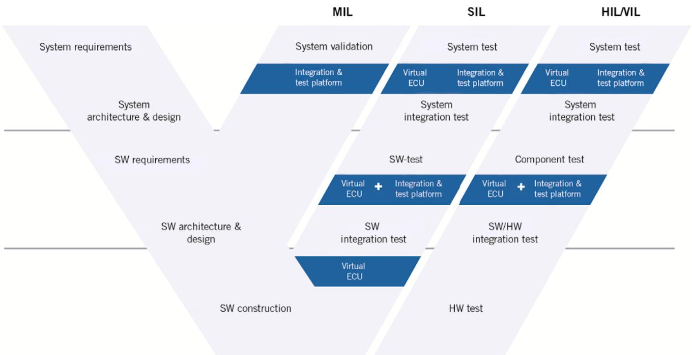
**FIGURE 1** Visualisation of the use of virtual ECU testing in an integration and test platform for the various development stages of a full vehicle (V-process)
