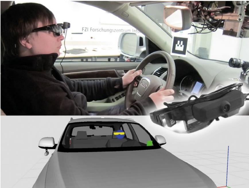
4 Test drive with augmented reality glasses (top) and head posture recognition visualised in the virtual model (bottom)
