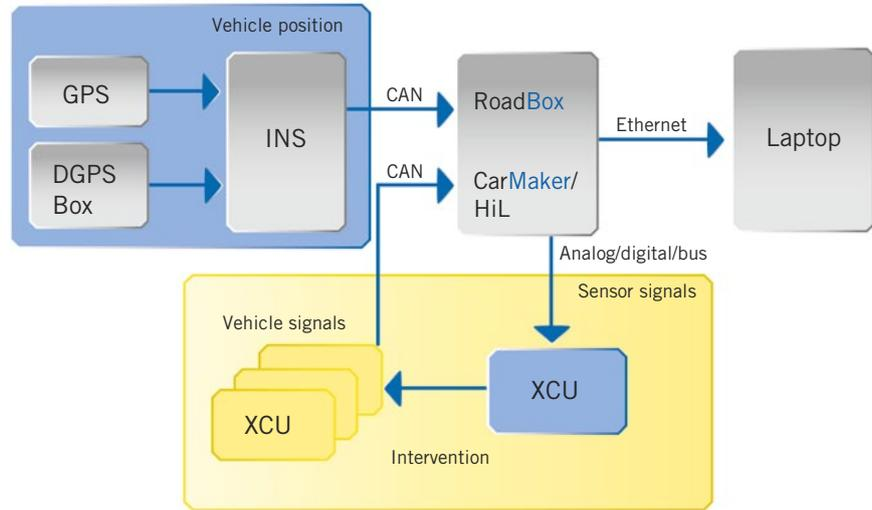
3 Schematic representation of the functional principle of a ViL configuration
