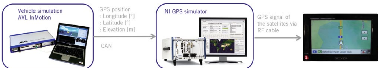
⑤ Simplified system structure consisting of a real-time system with the vehicle simulation AVL InMotion, the NI GPS simulation system and a portable navigation device
