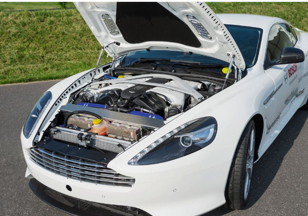
4 Aston Martin DB9 concept car with axle-split hybrid powertrain
