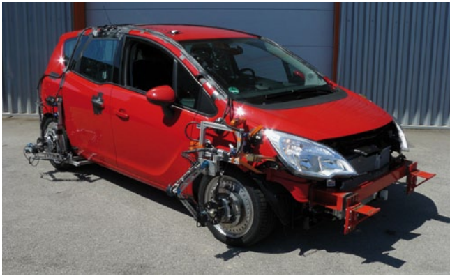
2 The Opel Meriva reference vehicle with Idiada instrumentation for dynamic driving tests
