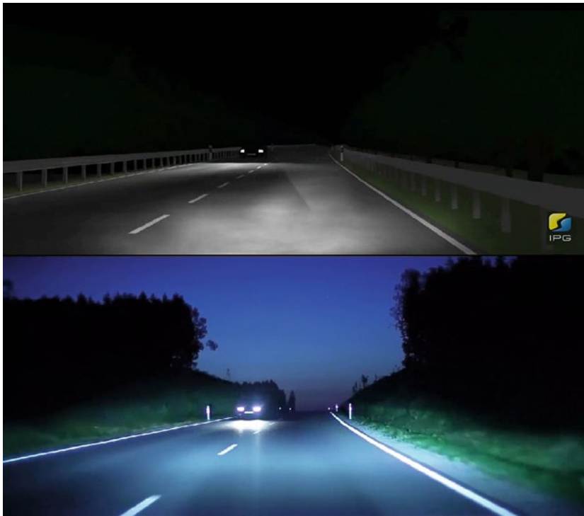
4 Comparison of the light function: video (below) with glare-free high beam and its simulation (above)
