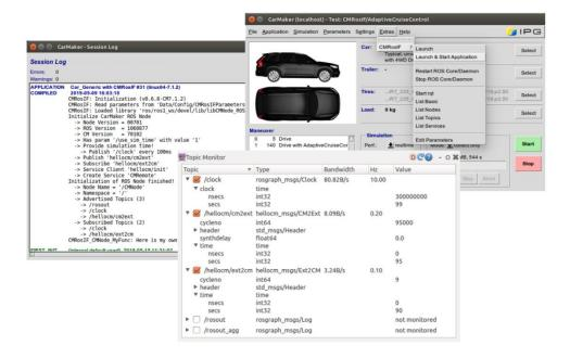
The demo package provides an example that demonstrates a basic communication between a ROS Node inside CarMaker and an external ROS Node with or without a simple synchronization mechanism.
