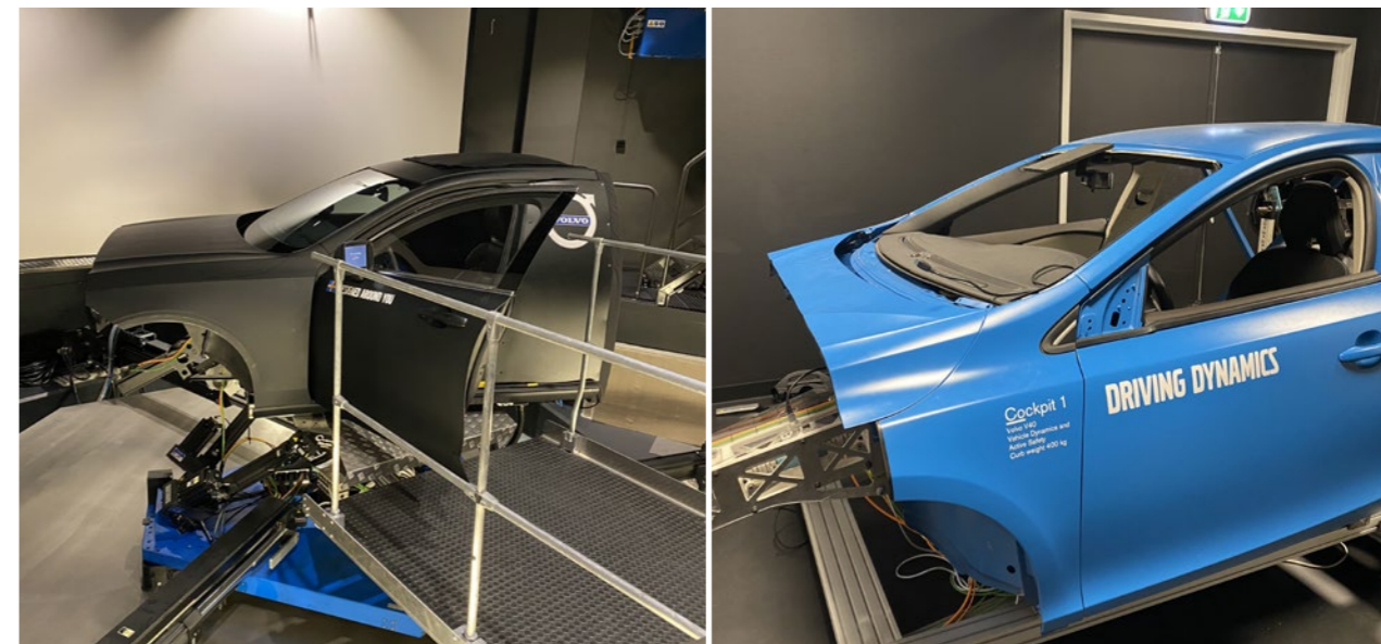
The dynamic driving simulator (black) and the static driving simulator (blue) at Volvo Cars in Gothenburg.
