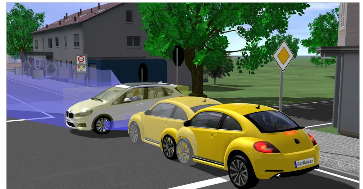
Figure 3: Comparison between an ideal and a phenomenological radar sensor model
