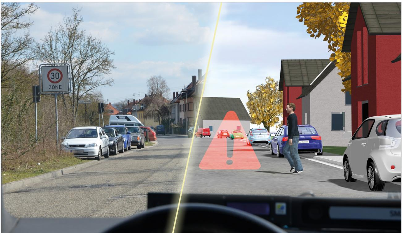
Testing an emergency brake assist system with the vehicle-in-the-loop method
