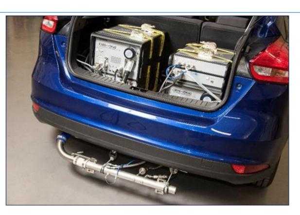
EXHAUST SYSTEM Exhaust gas mass flow
