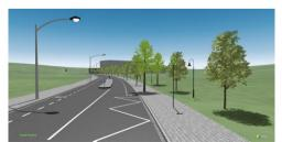
Export of the precise as-built-plan into Road5 Format for IPG CarMaker, which can directly be used for customer applications.
