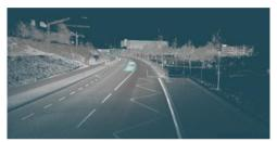
Object information extraction on the basis of camera and scanner data, e.g. traffic signs, markings, guide posts etc..
